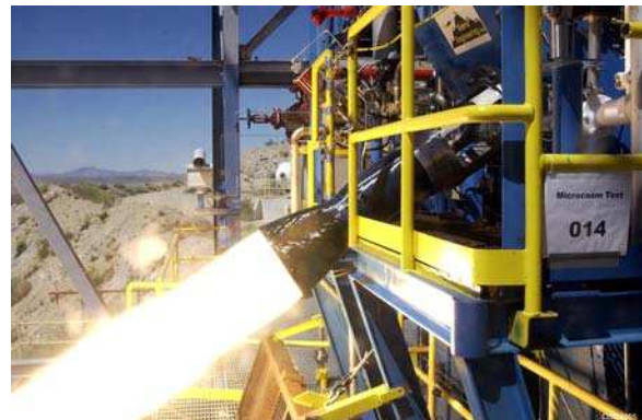
Figure 6: 20K lb f Engine Firing with Flight-type Chamber.
