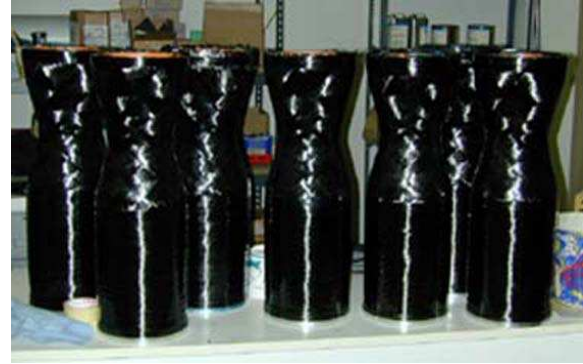
Figure 2: 5K lb f Thrust Chambers.
