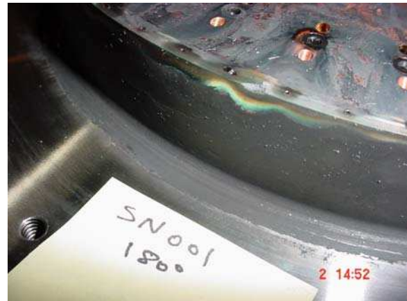
Figure 8: Close-up of Pit on Injector Lip Associated with Remanufactured FFC Orifice.
